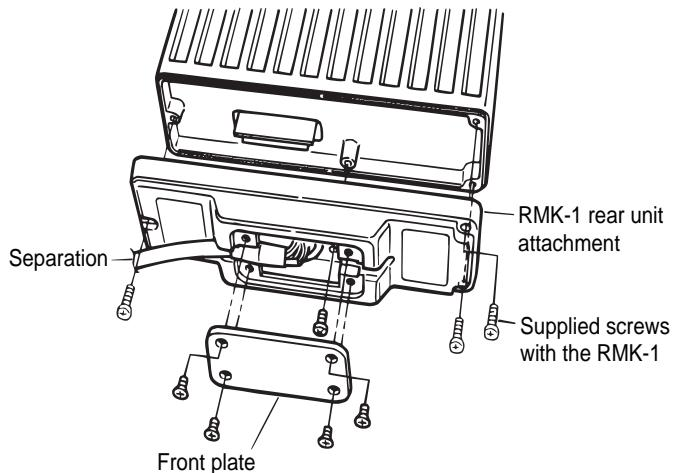
⑦ Remove 4 screws from the 'RMK-1 front unit attachment' to open the rear plate.
