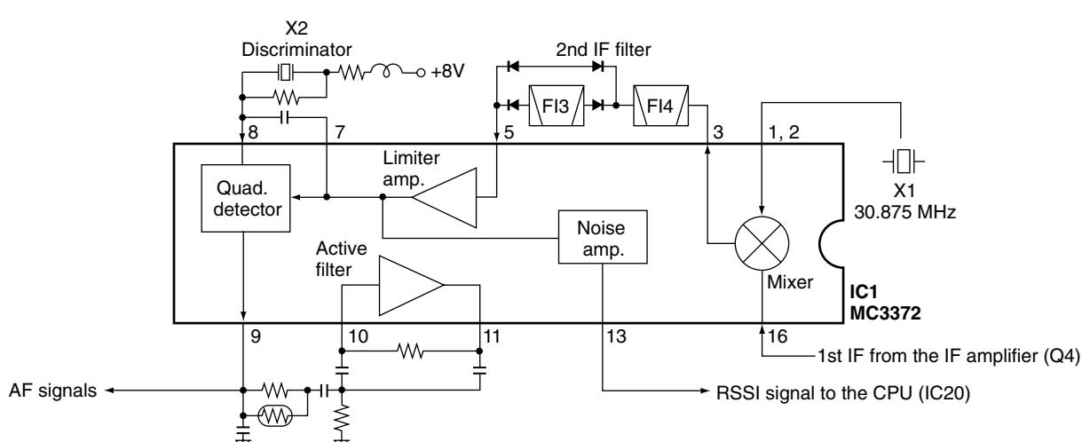
The N/W switches (D501, D502) select a ceramic filter (FI3 or bypass), and the other N/W switch (Q61) adjusts the input level of the FM IF IC (IC1, pin 8) to switch the bandwidth depending on the NWC signal from the CPU (IC20, pin 57). When NWC signal becomes high level, bandwidth setting is wide.
